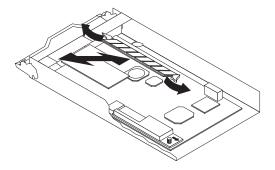
Figure 55. Installing the DIMM in the controller
